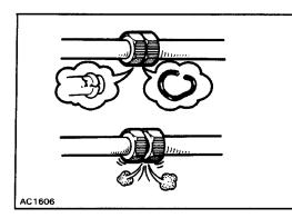
• Tighten the O-ring fittings or the bolted type fittings to the specified torque.
