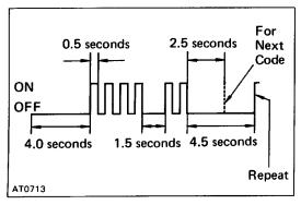
In the event of a malfunction, the light will flash 1 time per second. The number of blinks will equal the first number and, after 1.5 seconds pause, the second number of the two digit diagnostic trouble code. If there are two or more codes, there will be a 2.5 seconds pause between each.
