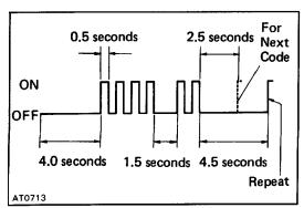
In the even of a malfunction, the light will flash 1 time per second. The number of blinks will equal the first number and, after 1.5 seconds pause, the second number of the two digit diagnostic trouble code. If there are two or more codes, there will be a 2.5 seconds pause between each.
