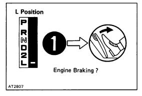
(b) While running in the L position, release the accelerator pedal and check the engine braking effect.
