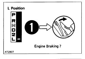
(b) While running in the L position, release the accelerator pedal and check the engine braking effect.
