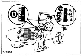
(b) When the transfer lever is shifted from H4 to L4, confirm that the gear changes according to the shifted diagram (See page AT-141). If it does not, the No.4 solenoid, ECM or transfer faulty.
