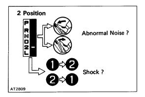
(c) Check for abnormal noise at acceleration and deceleration, and for shock at up-shift and down-shift.
