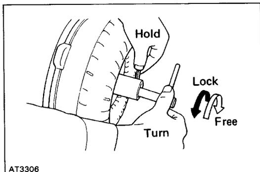
(c) With the torque converter clutch standing on its side, the clutch locks when turned counterclockwise, and rotates freely and smoothly clockwise. If necessary, clean the converter and retest the clutch. Replace the converter if the clutch still fails the test.
