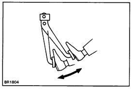
(d) Clear the diagnostic trouble codes stored in ECU by depressing the brake pedal 8 or more times within 3 seconds.
