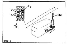
(c) Using SST, connect the terminal Tc to E, of the data link connector 1.
