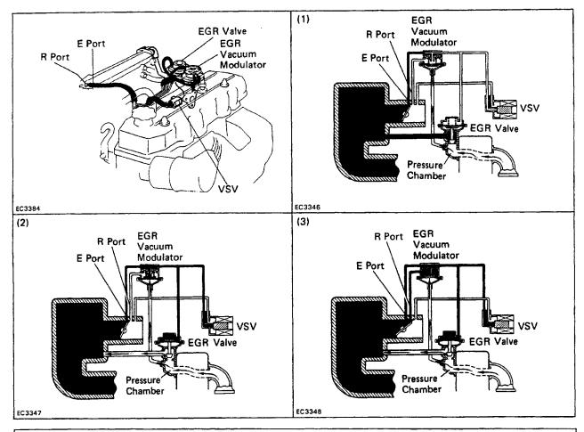
To reduce NOx emission, part of the exhaust gases are recirculated through the EGR valve to the intake manifold to lower the maximum combustion temperature.
