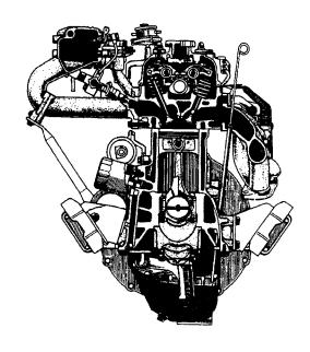
EM5984 EM5985 The 22R–E engine is in–line 4–cylinder engine with the cylinders numbered 1–2–3–4 from the front. The crankshaft is supported by 5 bearings inside the crankcase. These bearing are made of kelmet.
