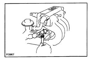
(c) When the pressure regulator fuel return hose (shown in the illustration at left), is pinched, the pressure within the high pressure line will rise to approx. 392 kPa (4 kgf/cm<sup>2</sup>, 57 psi). In this state, check to see that there are no leaks from any part of the fuel system.
