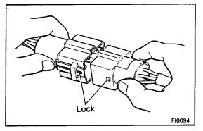
(b) Fully insert the connector and check that it is locked.
