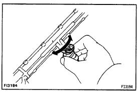
(c) Make sure that the injectors rotate smoothly. HINT: If the injectors do not rotate smoothly, the O-rings are probably incorrectly installed. Replace the O-rings.
