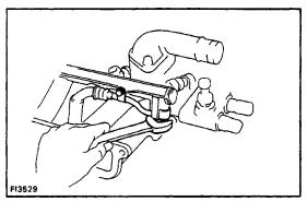
**5. DISCONNECT FUEL HOSE FROM DELIVERY PIPE** Remove the bolt, union bolt and two gaskets.
