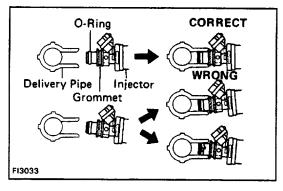
(b) Apply a light coat of gasoline to the O-rings and install the injectors into the delivery pipe.
