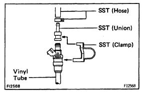
(d) Install SST (Union) to the injector and hold the injector and union with SST (Clamp).
