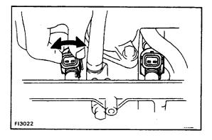
(c) Make sure that the injectors rotate smoothly.
