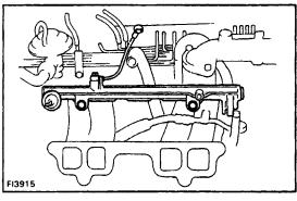
6. REMOVE DELIVERY PIPE WITH INJECTORS
