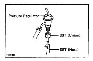
(c) Install SST (Union) to the removed pressure regulator. SST 09268–41045 (09268–52010)
