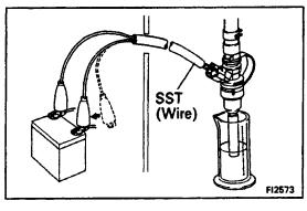
Connect SST (wire) to the injector and battery for 15 seconds and measure the injection volume with a graduated cylinder. Test each injector two or three times.
