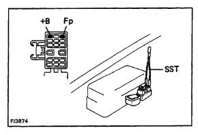
(h) Using SST, connect terminals Fp and +B of the DLC1. SST 09843–18020
