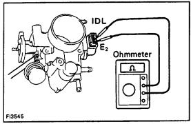
(b) Insert a thickness gauge (0.70 mm or 0.0276 in.) between the throttle stop screw and lever, and connect the ohmmeter to terminals IDL and E2.
