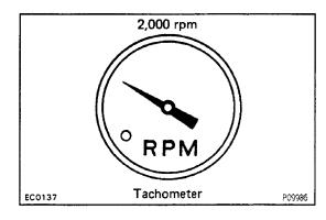
(c) Release the throttle valve.(d) Check the DP is set.DP setting speed: 2,000 rpm
