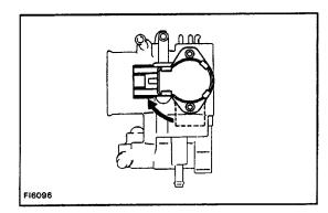
(c) Gradually turn the sensor clockwise until the ohmmeter deflects, and secure the sensor with the two screws.
