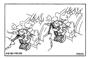
(e) If not as specified, adjust with the throttle opener adjusting screw.
