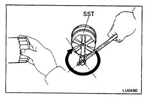
(d) Tighten the filter by hand until the gasket contacts the seat of the filter mounting. Then using SST, give it an additional 3/4 turn to seat the filter. SST 09228–07500
