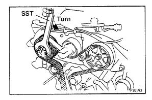
(a) Using SST, loosen the tension spring between the LH and RH camshaft timing pulleys by slightly turning the LH camshaft timing pulley clockwise.
