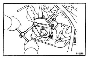
Remove the three bolts, timing belt cover and gasket.
