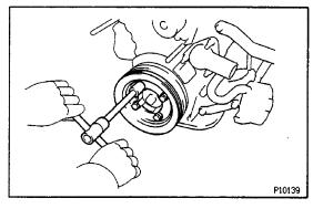
(d) Install the PS drive belt pulley with the four bolts.
