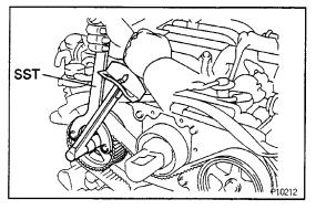
(f) Using SST, install the pulley bolt. SST 09278–54012
