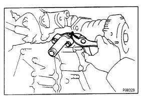
(c) Using pliers, remove the 1.5 mm hexagon wrench from the belt tensioner.
