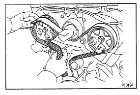
(b) Disconnect the timing belt from the camshaft timing pulleys.
