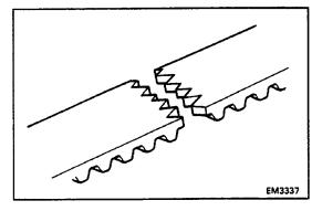
(b) If the belt teeth are cracked or damaged, check to see if either camshaft or water pump is locked.
