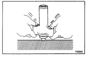
(b) Hold the tensioner with both hands, and push the push rod firmly against the floor or wall to check that it doesn't move.
