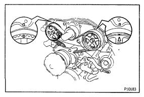
(b) Check that the timing marks of the camshaft timing pulleys and No.3 timing belt cover are aligned. If not, turn the crankshaft pulley one revolution (360°).
