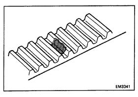
(e) If there is noticeable wear on the belt teeth, check the timing cover for damage, correct gasket installation, and foreign material on the pulley teeth. If necessary, replace the timing belt.
