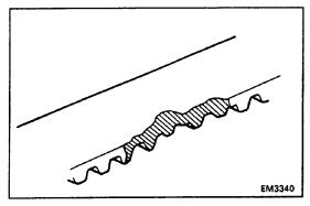
(d) If there is wear or damage on only one side of the belt, check the belt guide and the alignment of each pulley.
