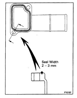
(c) Install the water outlet with the two bolts. Alternately tighten the bolts.Torque: 8.3 N-m (85 kgf-cm, 73 in.-lbf)
