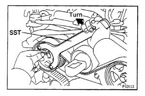
(e) Using SST, align the knock pin hole of the camshaft with the knock pin groove of the pulley and install the knock pin.
