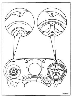
(b) (RH Camshaft Pulley Position)
