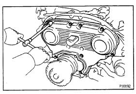
(c) Remove the eleven bolts, timing belt cover and three gaskets.
