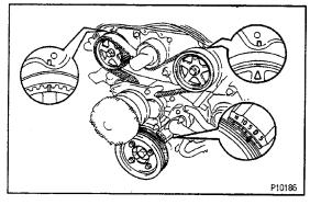
(b) Check that each pulley aligns with the timing marks as shown in the illustration.If the timing marks do not align, remove the timing
