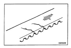
(c) If there is noticeable wear or cracks on the belt face; check to see if there are nicks on the side of the idle pulley lock.
