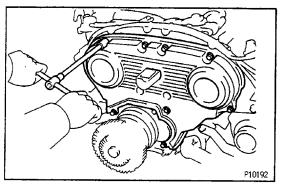
(d) Install the timing belt cover with the eleven bolts.
