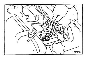
(t) Using two new gaskets, reconnect the No.3 fuel pipe to the delivery pipe.
