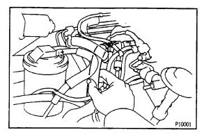
(c) Check that there is pressure in the fuel inlet hose. HINT: At this time, you will hear fuel return noise from the fuel return hose.
