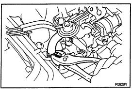
(d) Disconnect the No.4 water by–pass hose from the union of the intake manifold.
