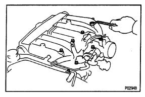
(q) Remove the six bolts, two nuts, intake chamber and gasket.
