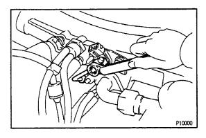
(m) Connect the cold start injector tube with new a gasket and the union bolt.
