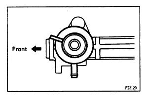
(d) Turn the fuel pressure regulator counterclockwise until the outlet faces in the direction indicated in the illustration.
