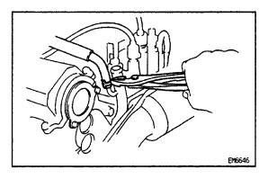
(e) Disconnect the No.5 water by–pass hose from the water by–pass pipe.
