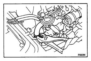
(p) Connect the No.4 water by–pass hose to the union of the intake manifold.
