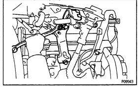
(k) Remove the nut, two bolts, intake chamber stay and throttle cable bracket.
