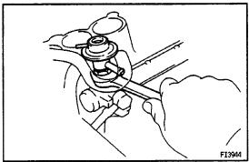
(e) Torque the lock nut.
