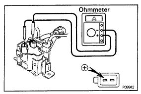
4. MEASURE SECONDARY COIL RESISTANCE Using an ohmmeter, measure the resistance between the positive (+) terminal and high-tension terminal. Secondary coil resistance (Cold):9.0 –15.4k $\Omega$ Secondary coil resistance (Hot) :11.4–18.1 k $\Omega$ 5. CONNECT HIGH-TENSION CORD
