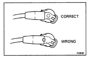
NOTICE: Check that the holder is correctly installed to the grommet and distributor cap as shown in the illustration.
