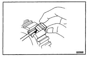
(b) Push the shifting key spring with screwdriver, remove the three shifting keys and key springs.
