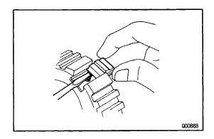
(b) Push the shifting key spring with screwdriver, remove the three shifting keys and key springs.
