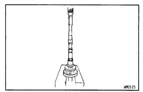
(c) Using a press, install the 3rd gear and No.2 clutch hub.
