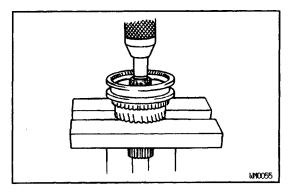
(b) Using a press, remove the No.2 hub sleeve, synchronizer ring and 3rd gear.
