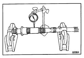
(e) Using a dial indicator, check the shaft runout.
