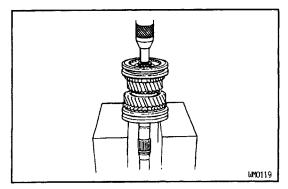
(d) Using a press, install the 2nd gear and No.1 clutch hub.
