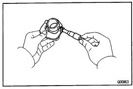
(d) Using a micrometer, measure the outer diameter of the inner race.
