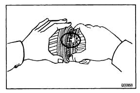
(d) Install the assembly on the output shaft with the synchronizer ring slots aligned with the shifting keys and turn the inner race to align it with the locking ball.
