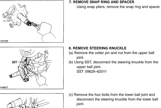
disconnect the steering knuckle from the lower ball
