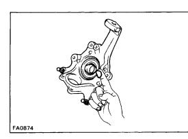
(c) Apply molybdenum disulphide lithium base grease to the steering knuckle bushings.
