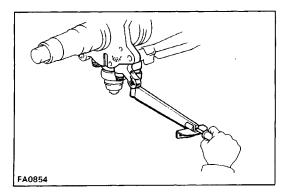
(c) Connect the lower ball joint to the steering knuckle and install and torque the four bolts.
