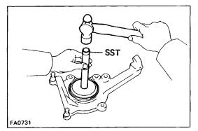
5. INSTALL DUST DEFLECTOR TO STEERING KNUCKLE Using SST and a hammer, tap in a new dust deflector. SST 09608–35014 (09608–06020, 09608–06180)
